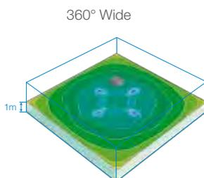
Temperature distribution by thermograph (cooling operation)
