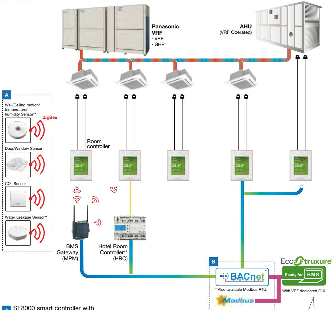
**A** SE8000 smart controller with direct hub to ZigBee® Pro sensors. Great Occupancy and IAQ control. Ex: Hotel room occupancy check by PIR sensor, IAQ by CO<sub>2</sub> sensor, Door / Window contacts.
