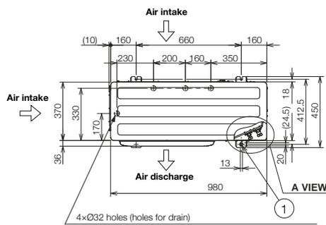
When using a drain pipe, install the drain socket (field supply) on to the drain port. Seal the other drain port with the rubber cap.
