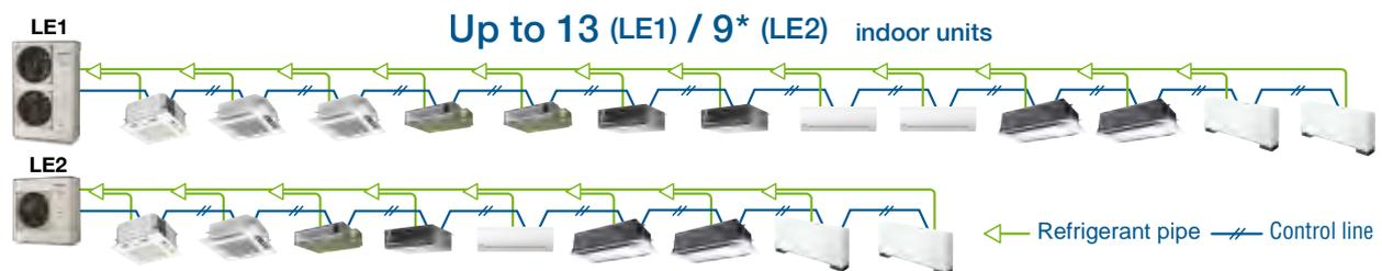
\* Use any of the 22 type indoor models. Depending on the size or type of indoor unit, tubing size shall be changed. Please refer manuals for details.
